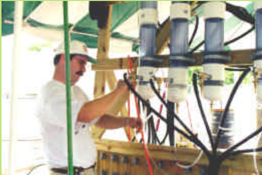
Mike Annable of the UF environmental engineering department taking groundwater samples to evaluate remediation efficiency at the Sages site.
