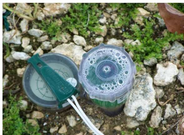
Figure 4. Switching tensiometer. Credits: H. Trafford
