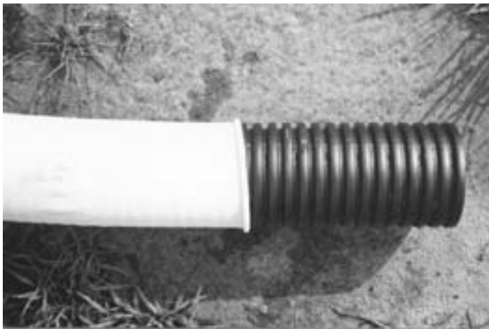
Figure 17. Four-inch corrugated drain tubing with polyester sock.
