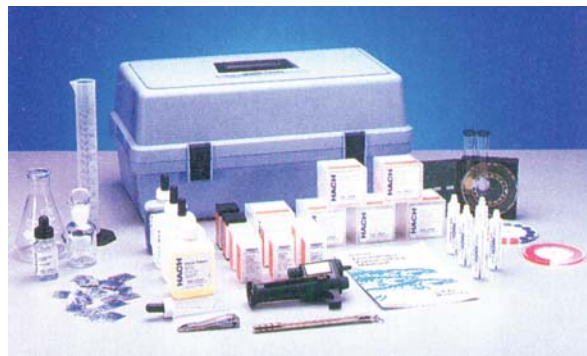
Figure 5. Field test kit for acidity, alkalinity, carbon dioxide, DO, hardness, and pH with color wheel and digital titrator.
