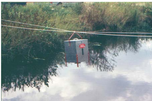
Figure 9. Turkey feeder used to periodically disperse fluridone pellets into a canal. Credits: L. Pell
