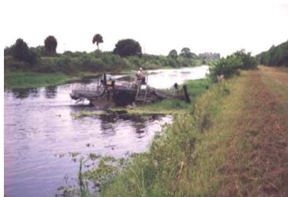
Figure 6. Mechanical aquatic weed removal from canal. Credits: P. Whalen
