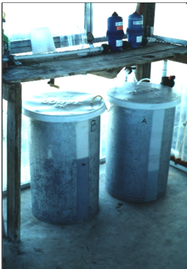
Figure 2. Stock tanks containing concentrated fertilizer are located under the fertilizer proportioner bench to conserve space.
