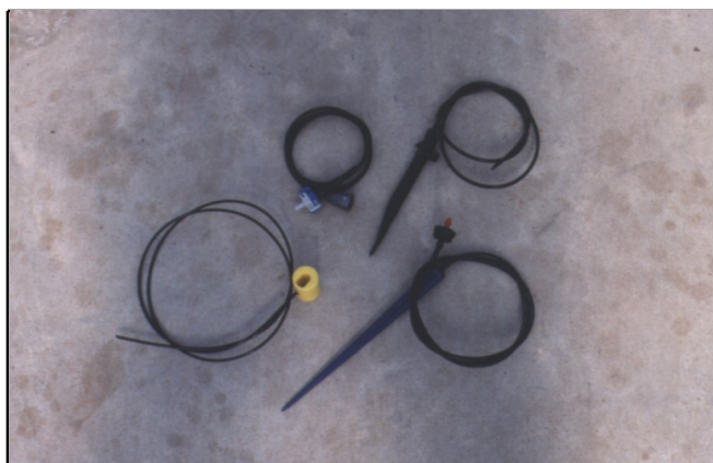
Figure 1. Several types of irrigation emitters for supplying nutrient solution to vegetable plants in bag, perlite, or rockwool culture.
