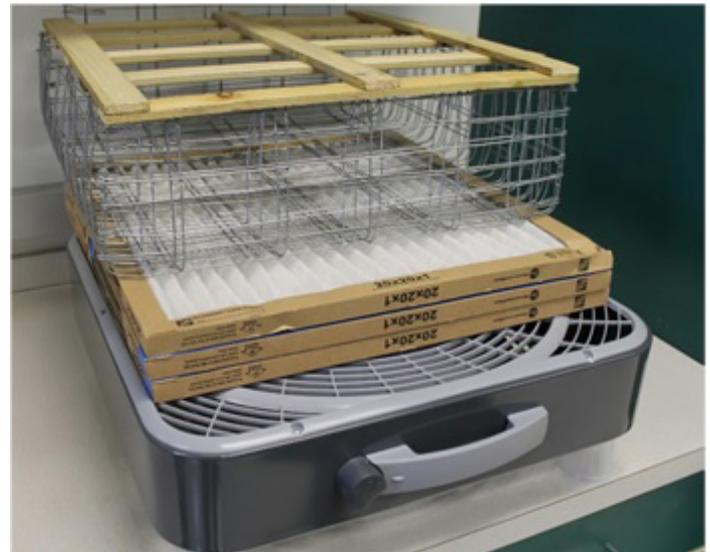
Figure 1. MREC drying rig, spread out to show the possible components. From top to bottom: modified wooden slat, 20x20" wire cage, 20x20x1" natural fiber household air duct filters, 20" box fan. Credits: Sean M. Campbell, UF/IFAS
