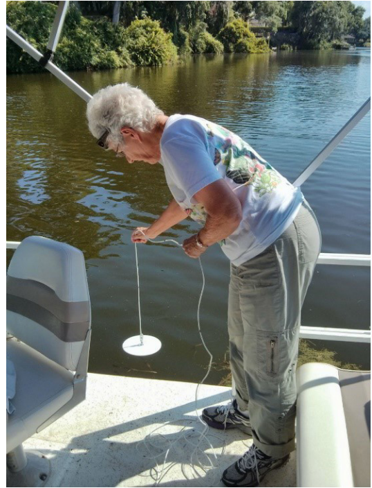
Figure 2. A Lakewatch volunteer in Lakeland, FL, demonstrates how to take a Secchi disk sample.
