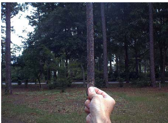
Figure 2. This tree will be included in the volume estimate. Note that the tree appears wider than the nickel angle gauge.
