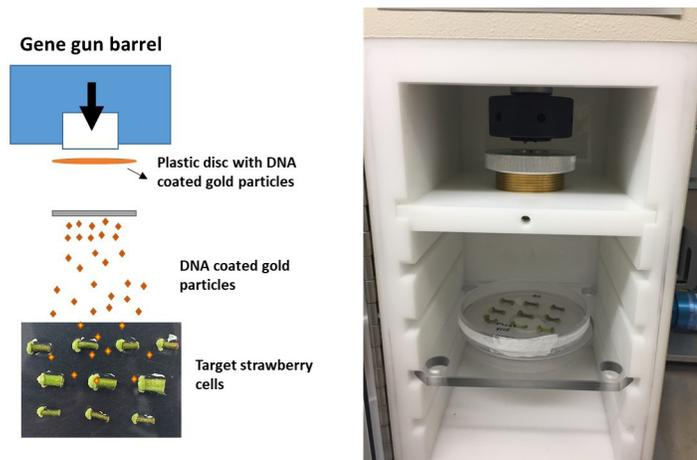
Figure 3. General procedure of transformation using the metal particle bombardment system.
