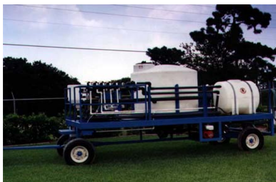
Figure 6. Portable mix-load stations with slurry tank and spray oil storage.
