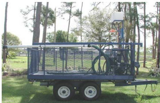
Figure 5. Portable mix-load stations designed for flatwoods grove with plumbing to access ditch water. This design has no oil or slurry tank.
