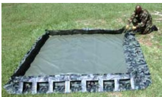
Figure 1. Pan containment system.
