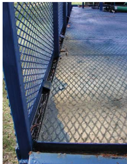
Figure 4. Closeup of guttering for spill containment in portable mix-load station.
