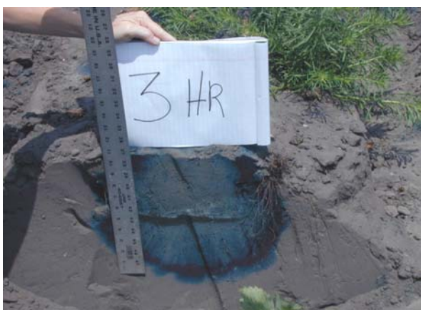
Figure 3. Cross section after 3 hours of irrigation. Credits: J.R. Duval 2002
