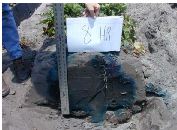
Figure 6. Cross section of beds after 8 hours. Credits: J.R. Duval 2002
