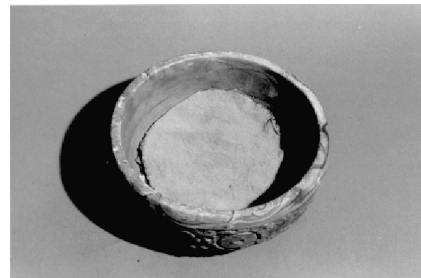
Figure 3. Cover the pea-size gravel with a piece of synthetic fabric.
