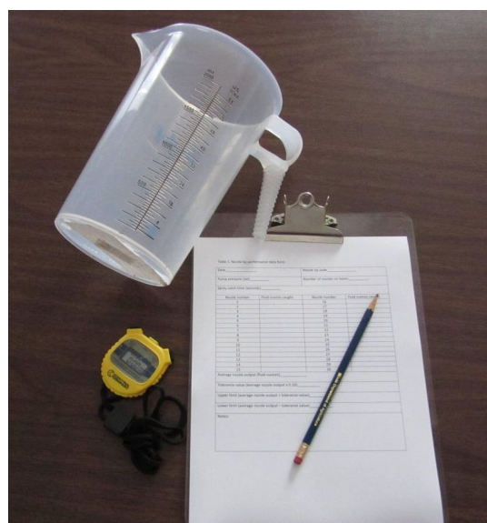
Figure 2. Simple items needed for performing a nozzle performance test. Photo credit: UF/IFAS Pesticide Information Office.
