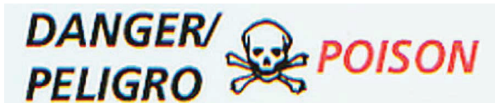
Figure 1. “POISON” and the skull-and-crossbones symbol should appear near the signal word “DANGER”.
