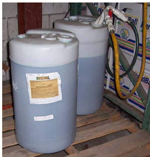
Figure 1. Closed Mixing and Loading System for Delivering Pesticide to the Application Equipment Credits: UF/IFAS Pesticide Information Office
