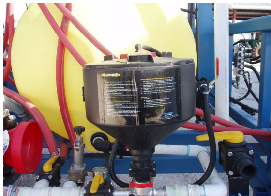
Figure 2. Commercial Loading System for Delivering Pesticide to the Spray Tank Credits: UF/IFAS Pesticide Information Office
