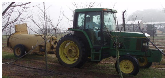
Figure 4. Enclosed cab of a tractor surrounds the pesticide applicator. Credits: UF/IFAS Pesticide Information Office
