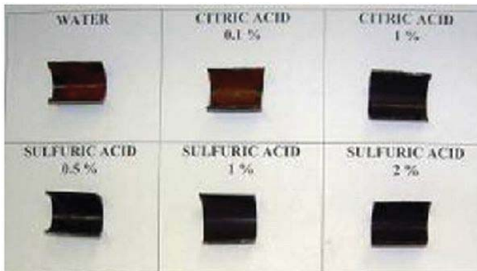
Figure 4. Treatment of iron scale formed within irrigation tubing with sulfuric acid, citric acid, and a proprietary product at selected concentrations. Iron scale on the inside of the tubing is evident by the reddish brown/rust color.
