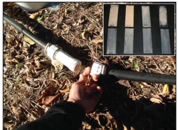
Figure 5. A 3/4-inch PVC coupling found in plumbing-supply stores serves well as in-line glass slide holder. Observing the amount, type, and rate of scale deposition occurring on a clean side (inset) can help determine the scaling potential of the irrigation water and the effect of injected scale-inhibiting chemicals.
