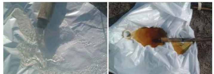
Figure 3. Flush water from treatment of scale using sodium hydrosulfite (left) and citric acid (right).
