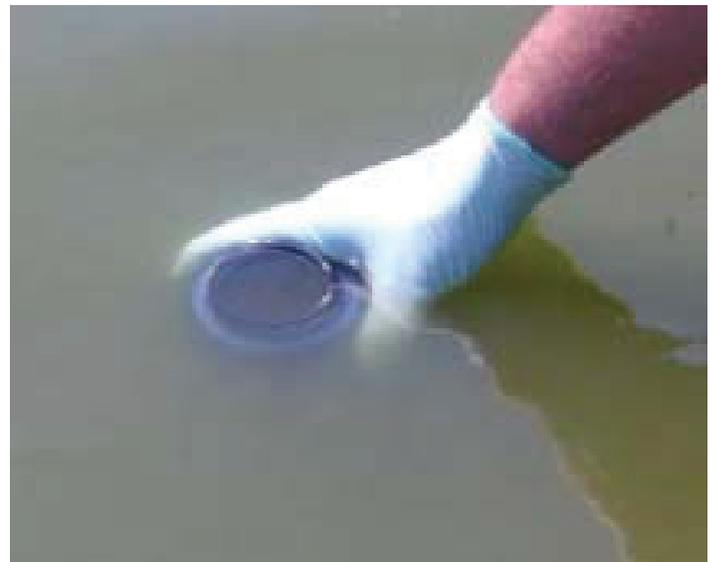
Figure 3. Seal under water to avoid trapping air.
