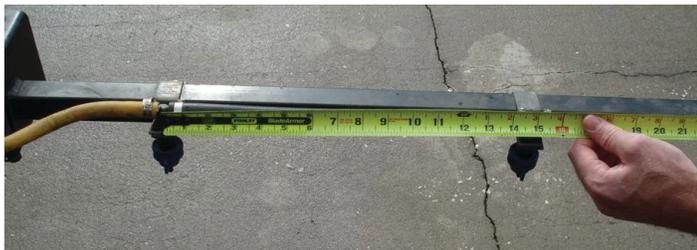
Figure 1. Measuring nozzle spacing to determine “W”.
