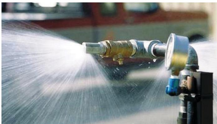
Figure 2. A wide-swath, boomless nozzle.
