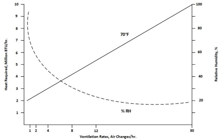
Figure 4. Heating required and inside relative humidity at 70°F as influenced by ventilation rate.
