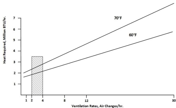
Figure 2. Heating requirement as influenced by inside temperature and ventilation rate.
