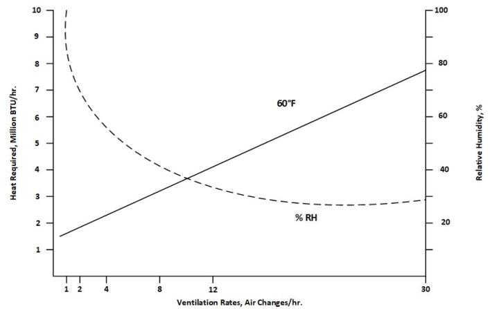
Figure 3. Heating required and inside relative humidity at 60°F as influenced by ventilation rate.
