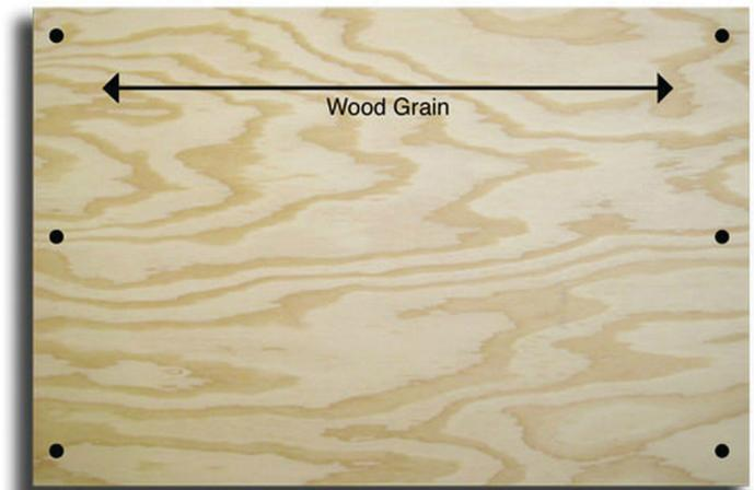
Figure 1. Plywood is strongest in the direction of its wood grain.
