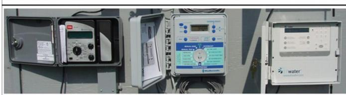
Figure 1. Photo of three brands of ET controllers from testing at the University of Florida, Agricultural and Biological Engineering Department.
