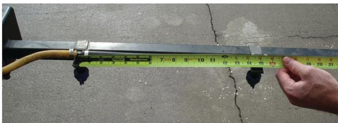
Figure 1. Measuring nozzle spacing to determine “W.”
