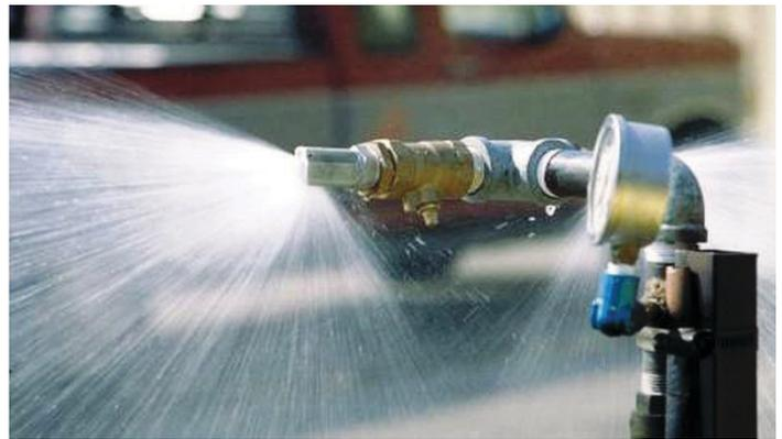
Figure 2. A wide-swath, boomless nozzle.
