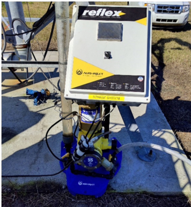
Figure 2. A fertigation-injector injects a liquid fertilizer into the irrigation water through the head of a center-pivot irrigation system. Credits: Xiangju Fu, UF/IFAS
