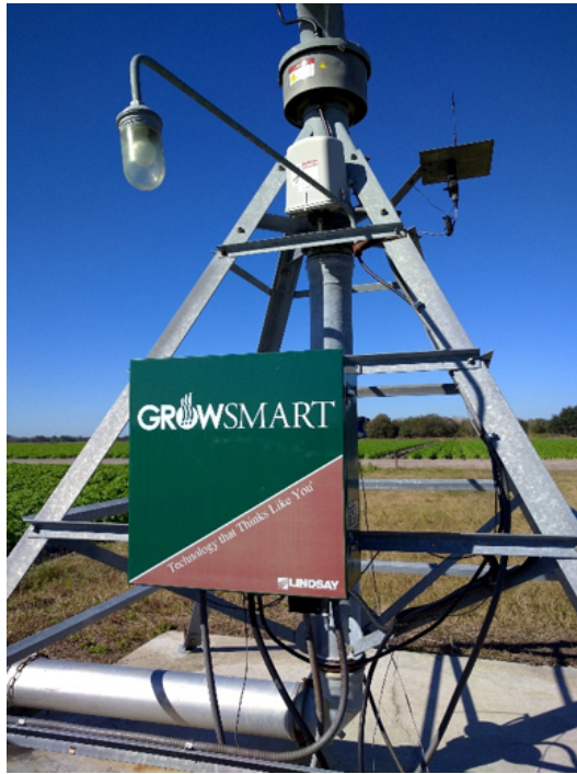
Figure 1. The head of a center-pivot irrigation system used for fertigation in southwest Florida. Credits: Xiangju Fu, UF/IFAS
