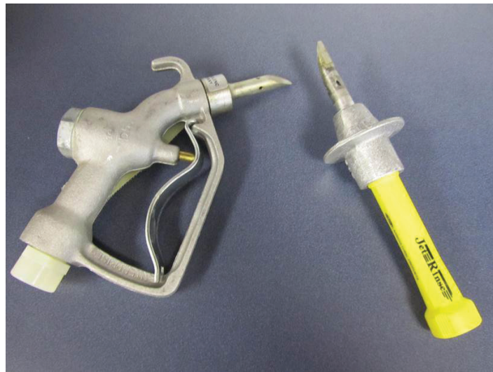
Figure 2. Varieties of pressure-rinse nozzles.
