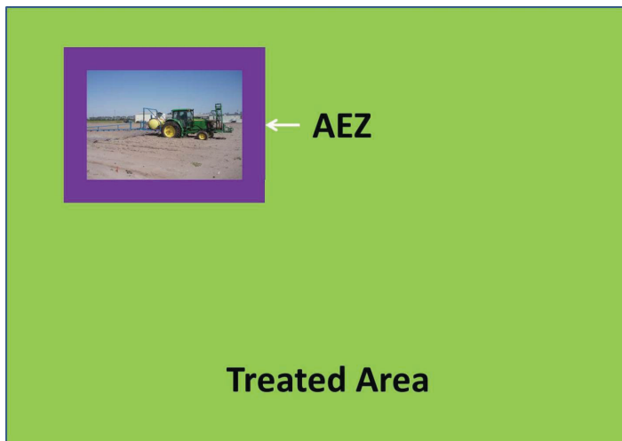
Figure 1. The AEZ is the purple area around the application equipment. It moves with the application equipment as it proceeds. The AEZ is generally within the treated area, except when the application equipment is near the edges of the treated area.
