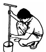
Figure 3. Place 10–15 soil cores into a plastic bucket; mix, dry, and transfer to a bag.
