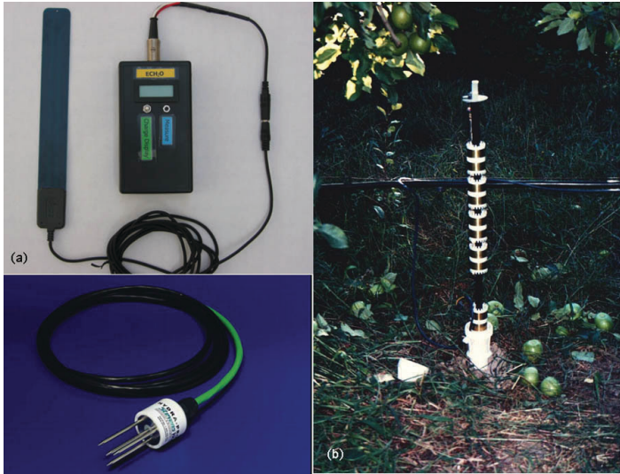
Figure 5. FD probes: a) Capacitance (plates imbedded in a silicon board); b) Capacitance (rods); and c) FDR (rings).
