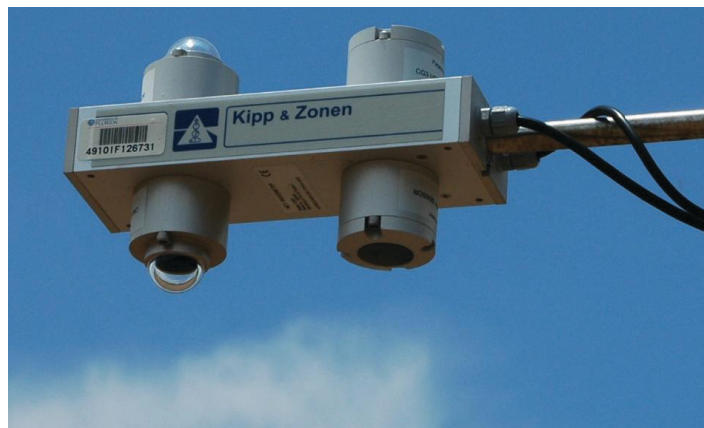
Figure 7. CNR-1 net radiometer. Credits: Calvin Tien, UF/IFAS
