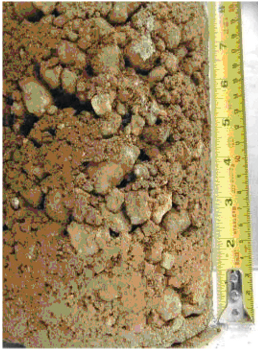
Figure 3. The shallow profile of Krome very gravelly loam at Homestead. This soil is only 8 inches deep and is underlain by limestone rock (not shown). Credits: Y. Li
