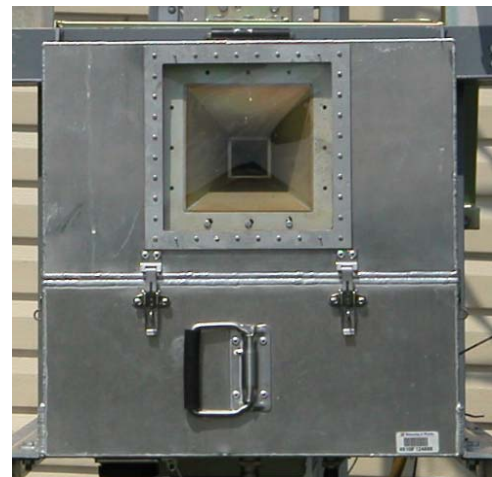
Figure 4 (b) and (c). The side view of the UFCMR showing the rotary system and the front view of the UFCMR showing the receiver antenna.
