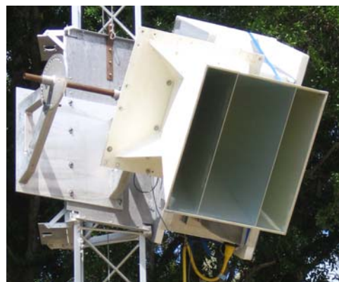
Figure 6 (b) and (c). The side view of the UFLMR showing the rotary system and the front view of the UFLMR showing the receiver antenna.
