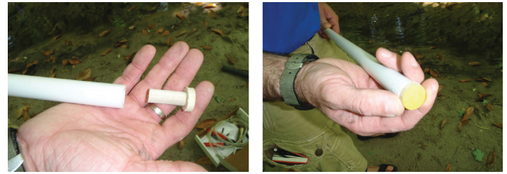
Figure 3. Mini-piezometer cap constructed from two sections of wooden dowels glued together. Credit: Shantih Spanton
