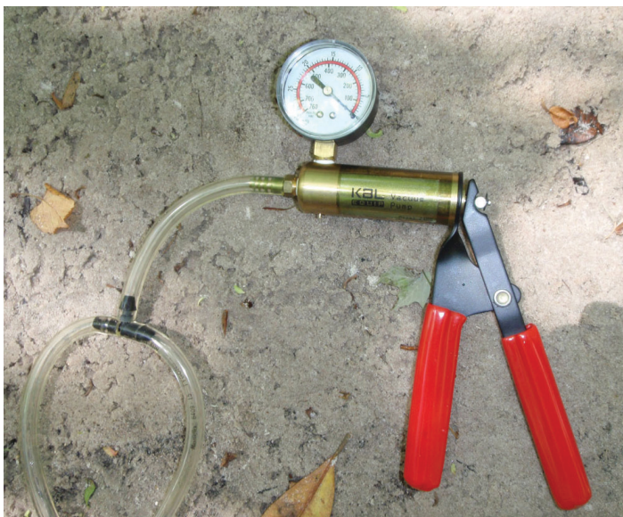
Figure 5. Hand vacuum pump connected to the T-Connector.
