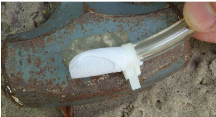
Figure 2. Nylon stocking used as filter fabric to prevent clogging of the perforations in the clear tube. Credit: Shantih Spanton
