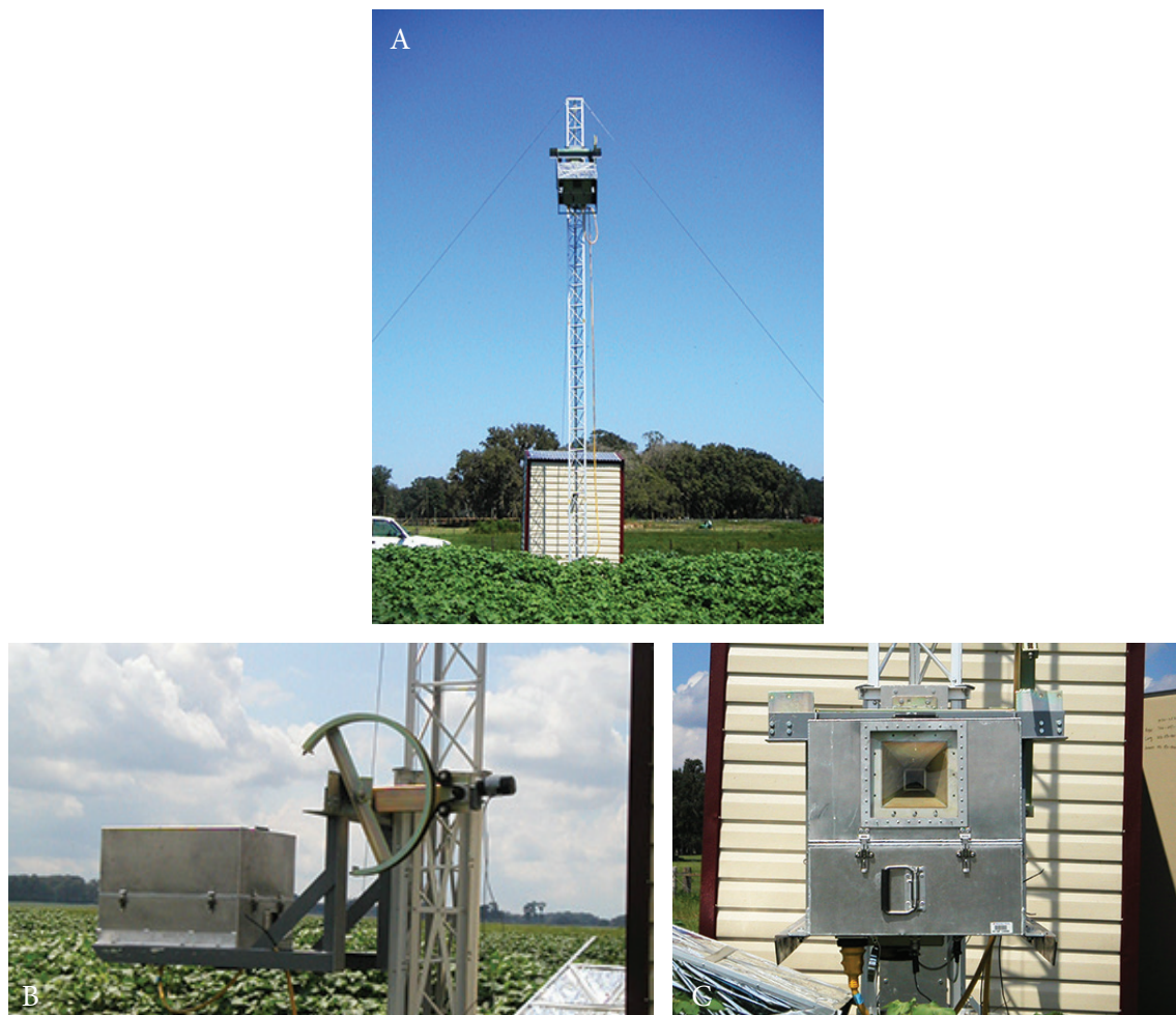
Figure 4. (a) The UFCMR system, (b) the side view of the UFCMR showing the rotary system, and (c) the front view of the UFCMR showing the receiver antenna.
