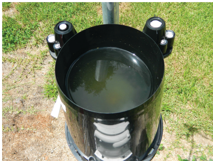
Figure 3. Most common problem found in rain gauges is clogging of the catchment funnel by insects, turf clippings, and dirt. Check weekly or more often if necessary.
