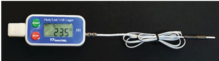
Figure 3. Data recorder with temperature sensor. Credits: Lauren Douma, UF
