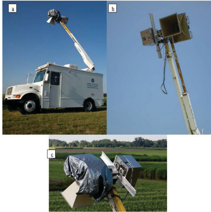
Figure 8. (a) The TMRS-L; (b) the front view of the TMRS-L showing the receiver antenna; and (c) the side view of the TMRS-L showing the rotary system.
