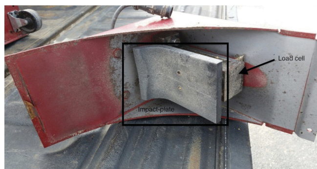
Figure 2. Flat impact-plate sensor taken out of a Case IH AF 6140 combine and turned on its side. Black rectangle indicates the impact plate. The black arrow points to the load cell behind the plate that converts pressure to voltage. Credits: Rebecca Barocco, UF/IFAS
