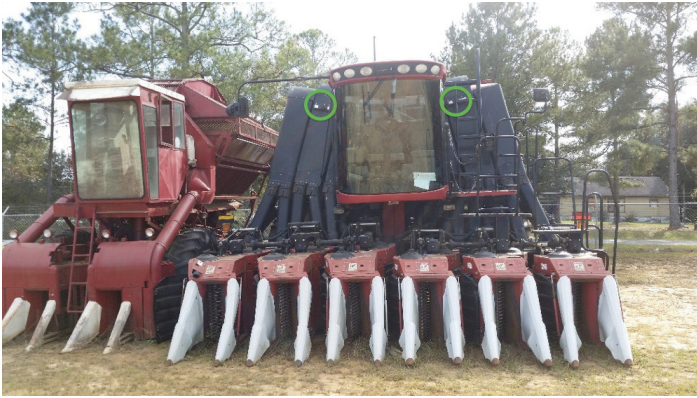
Figure 7. Location of optical sensor housing cut into the pneumatic ducts on a Case IH cotton picker (circled in green). Credits: Rebecca Barocco, UF/IFAS
