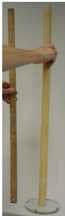
Figure 3. Schematic of soil chamber with CS616 sensor.
