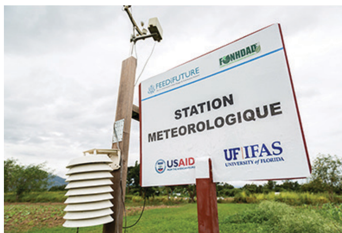
Figure 1: Example of a farm-based weather station established under an existing UF/IFAS project.
