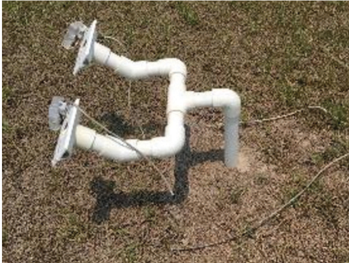
Figure 6. LWS mounting built with PVC pipe. Credits: T. B. Onofre, UF/IFAS
