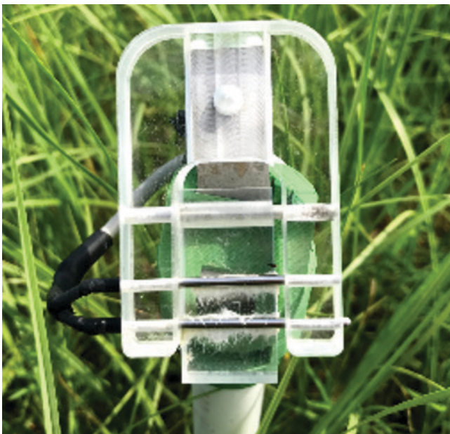
Figure 7. LWS with a missing paper. Credits: T. B. Onofre, UF/IFAS
