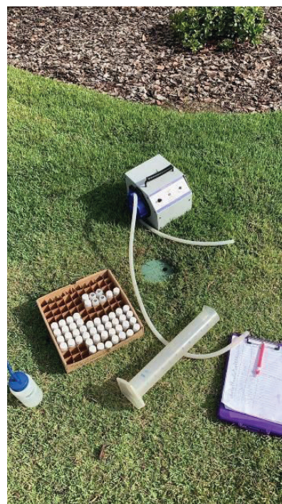
Figure 11. Equipment and supplies for leachate sample collection, including battery-powered peristaltic pump, graduated collection container, rinse bottle with deionized water for decontamination, sample collection bottles, and field sheet for recording leachate volumes. Credits: Jovana Radovanovic, UF/IFAS
