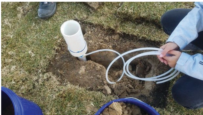
Figure 5. A notch for the collection tube is made and the lysimeter is ready for pea gravel.
