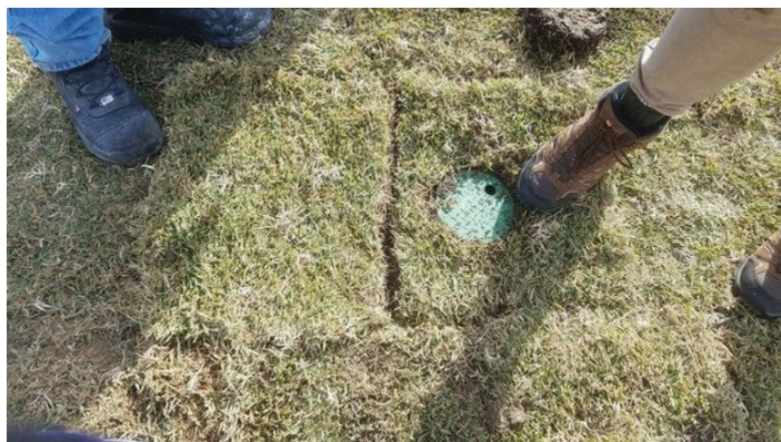
Figure 10. The turfgrass removed before installation was replaced over the lysimeter. An area was cut out of the sod to access the tube housing. Credits: Jovana Radovanovic, UF/IFAS
