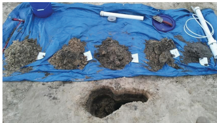
Figure 4. Each lift of soil is placed separately on a tarp and labeled to rebuild the soil profile later.
