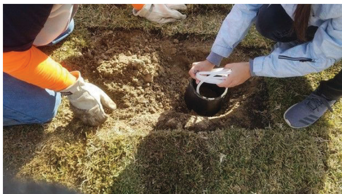
Figure 9. The soil profile is rebuilt, the access box is installed, and the collection tube is being rolled to be placed into the access box. Credits: Jovana Radovanovic, UF/IFAS
