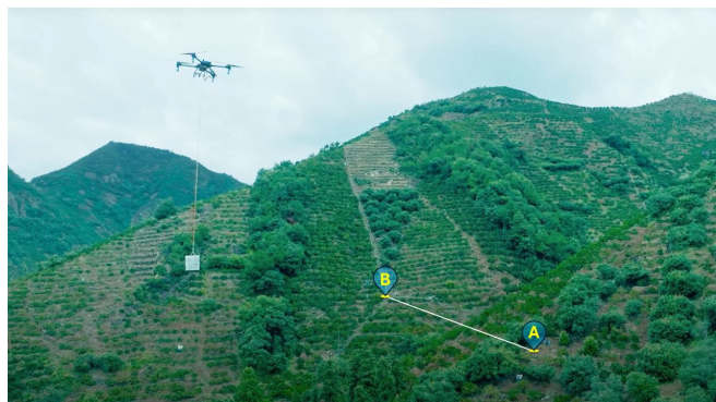
Figure 4. A spraying drone equipped with a cargo hoisting system transporting harvested fruit from the harvesting point (B) to the collection point (A).
