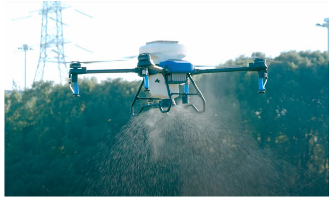
Figure 3. Spraying drone performing seeding with dry tank and spreader.
