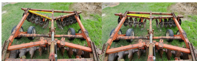
Figure 2. Heavy disk harrow with large (left) or small (right) gang angle, indicated by the yellow lines. A large angle increases disk penetration on soil and tillage and is used for preparing the soil. A small angle can be used for pushing rhizomes or stolons into the soil without covering them excessively.
