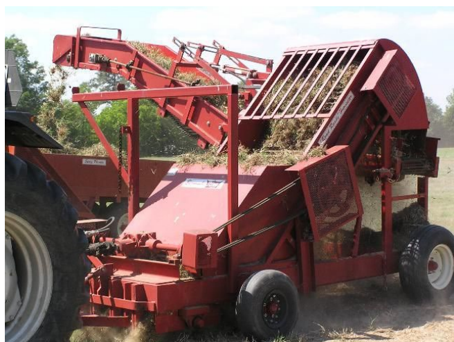
Figure 3. Sprig digger for bermudagrass. Credit: João Vendramini, UF/IFAS
