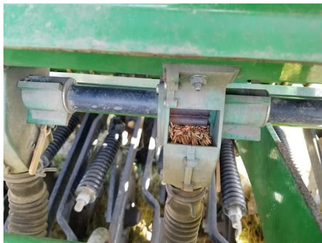
Figure 5. Oat and ryegrass seeds mixed in the main seedbox. Smaller ryegrass seed increases the speed of the flow compared to oat only.
