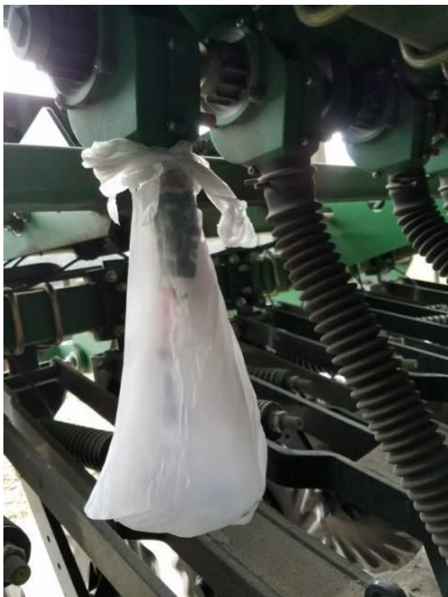
Figure 1. Remove the corrugated tube and attach a bag below the drive gear to collect the seeds. Credit: Marcelo Wallau, UF/IFAS
