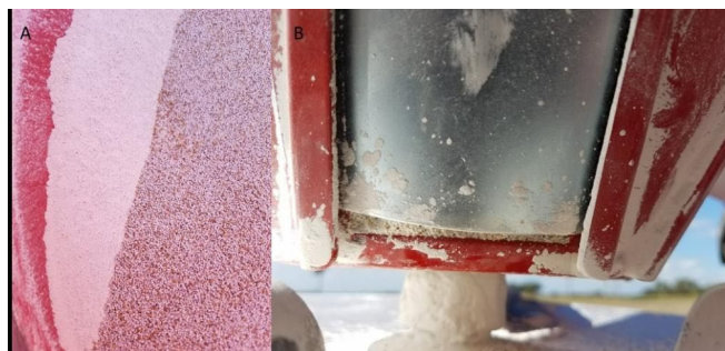
Figure 6. Coating material separated from white clover seeds (A) and clogging the seed gate (B).
