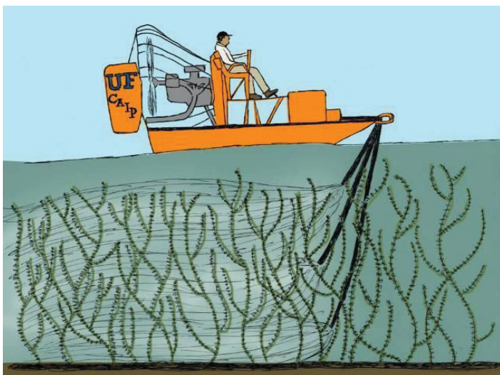
Figure 2. Whole water column treatment with trailing weighted hoses of various lengths. This figure shows herbicide discharging from the ends of the hoses, but it is actually released approximately 18" above the ends of the hoses (see text).
