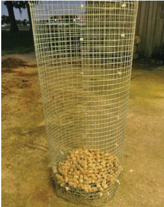
Figure 10. Hardware cloth basket designed to hold peanuts for blasting.
