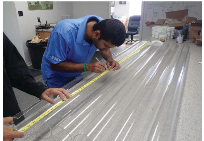
Figure 3. Clear acrylic tubes to be cut at 4-ft lengths. Credits: Cropping System Lab, UF/IFAS
