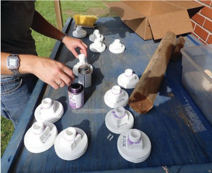
Figure 10. The repair coupling is glued to the threaded cap for the top section of the siphon. Credits: Cropping System Lab, UF/IFAS
