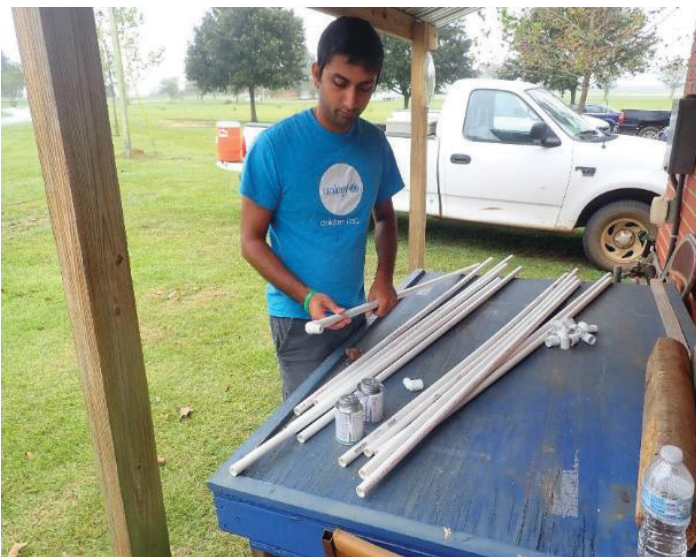
Figure 22. Elbow fitted to the air tube with primer and PVC glue. Credits: Cropping System Lab, UF/IFAS
