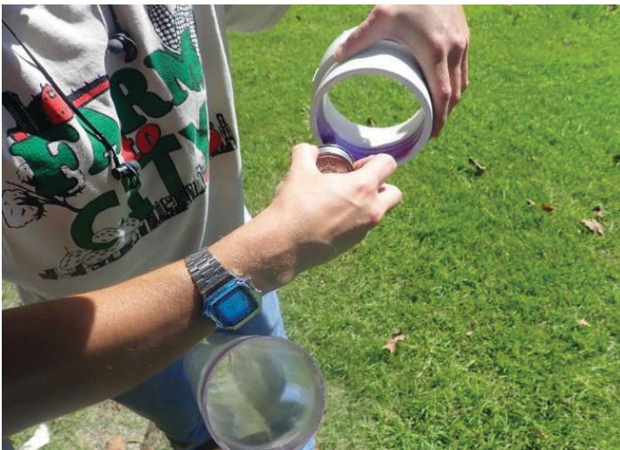
Figure 11. A 4-inch slip thread adapter is glued to the top of the clear acrylic tube and is later hammered into place with a rubber mallet for the bottom of the siphon. Credits: Cropping System Lab, UF/IFAS
