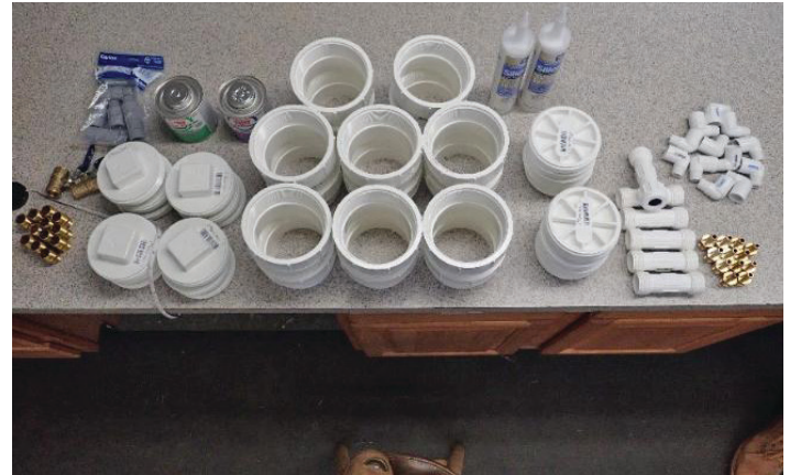
Figure 2. Assembly of fittings for the construction of multiple siphons. Credits: Cropping System Lab, UF/IFAS
