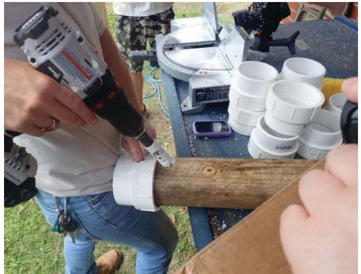
Figure 12. A 4-inch PVC slip thread adapter is drilled on the side using a hole saw (1 1/8-inch diameter) for the bottom of the siphon. Credits: Cropping System Lab, UF/IFAS
