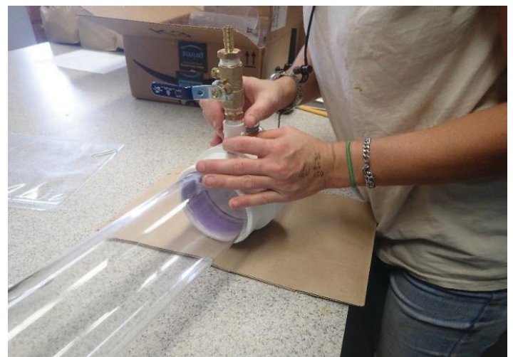
Figure 20. Assembled outlet port (riser, male adapter, brass ball valve, and brass barb) glued into bottom slip thread adapter.
