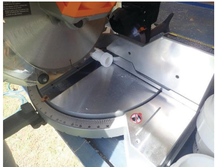
Figure 8. \frac{1}{2} -inch repair coupling is cut in half. Credits: Cropping System Lab, UF/IFAS
