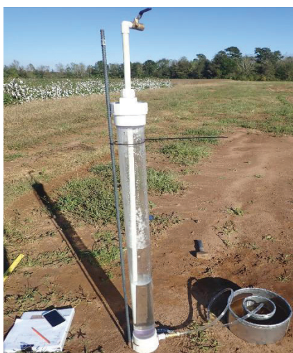
Figure 28. Mariotte siphon zip-tied onto a stand to produce constant head in a double ring infiltrometer to give accurate measurement of infiltration. The bottom of the air tube determines the height of the water column in the inner ring. Credits: Cropping System Lab, UF/IFAS
