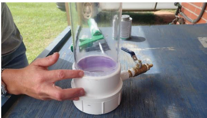
Figure 26. Silicone is applied at the top and bottom ends. Credits: Cropping System Lab, UF/IFAS
