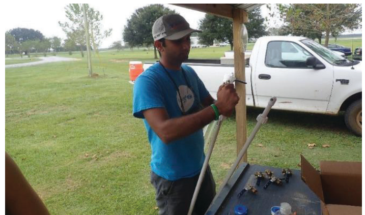
Figure 25. ½-inch brass ball valve screwed onto elbow at the top of the air tube. Credits: Cropping System Lab, UF/IFAS
