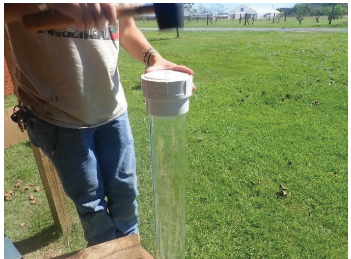
Figure 14. The bottom end of the siphon is glued and hammered into the acrylic tube with a rubber mallet. Credits: Cropping System Lab, UF/IFAS
