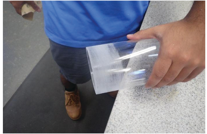
Figure 7. Both ends of the acrylic tube are sanded to about 5 cm on the outside of the tube. Credits: Cropping System Lab, UF/IFAS
