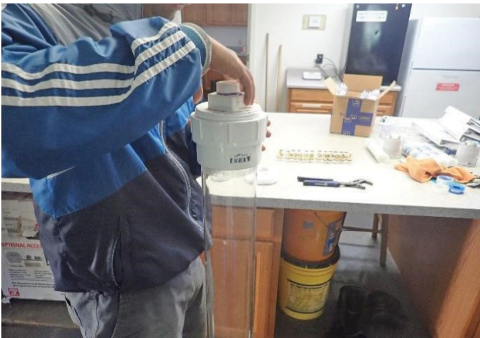
Figure 16. Assembled threaded cap is screwed into the 4-inch slip thread adapter for the top.
