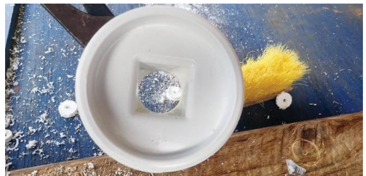
Figure 9. 4-inch threaded cap drilled using a hole saw ( 1\frac{3}{8} -inch diameter) for a \frac{1}{2} -inch repair coupling. Credits: Cropping System Lab, UF/IFAS
