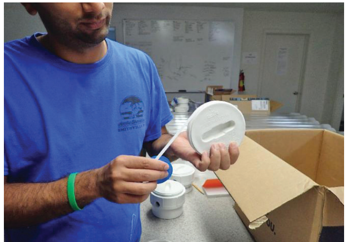
Figure 13. Teflon tape is added to the threaded PVC cap for the bottom of the siphon. Credits: Cropping System Lab, UF/IFAS
