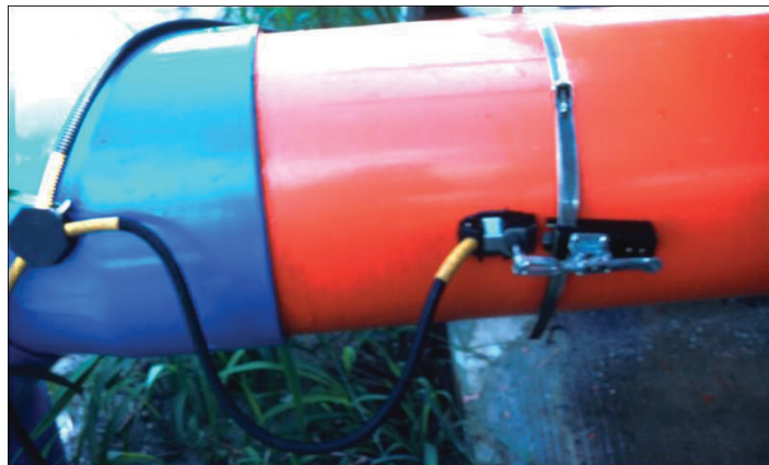
Figure 7. Transducers for ultrasonic flowmeter attached to 10-inch irrigation pipe
