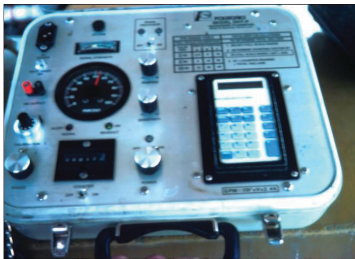
Figure 8. Transmitter and totalizing unit for ultrasonic flow meter.
