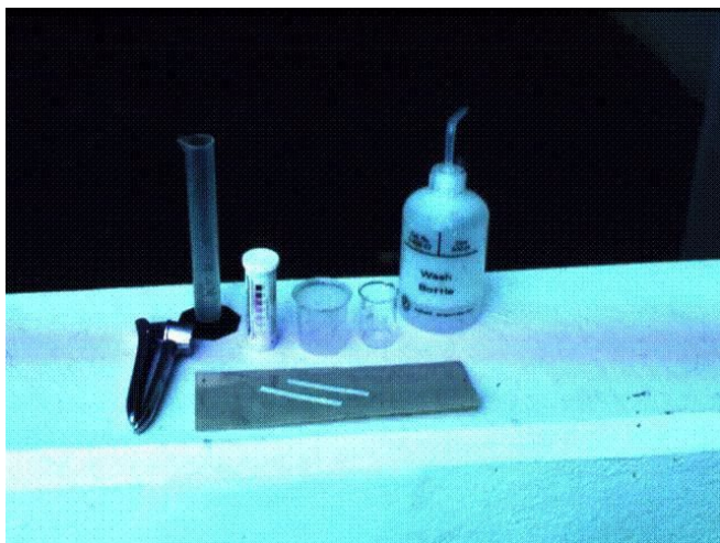
Figure 2. Testing petiole-sap using the MQuant strip test method.
