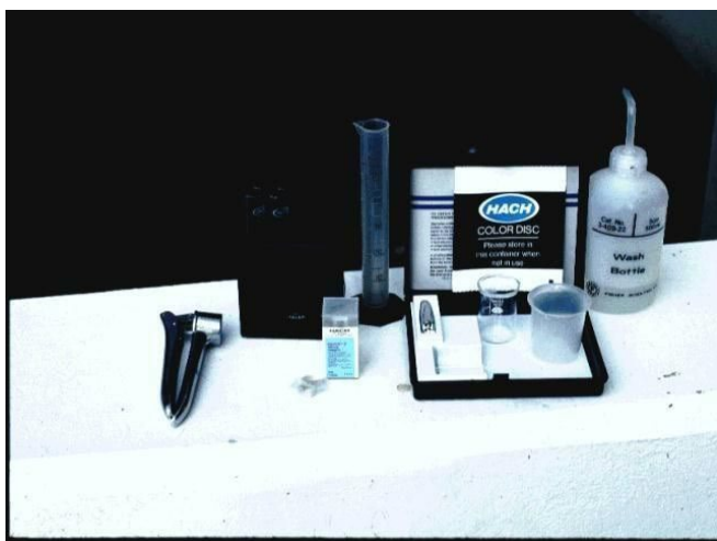
Figure 3. Petiole-sap testing using the Hach colorimeter test method.
