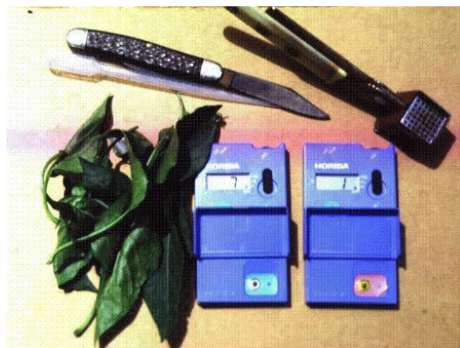
Figure 4. Cardy meters for Nitrate-N and K testing with samples.
