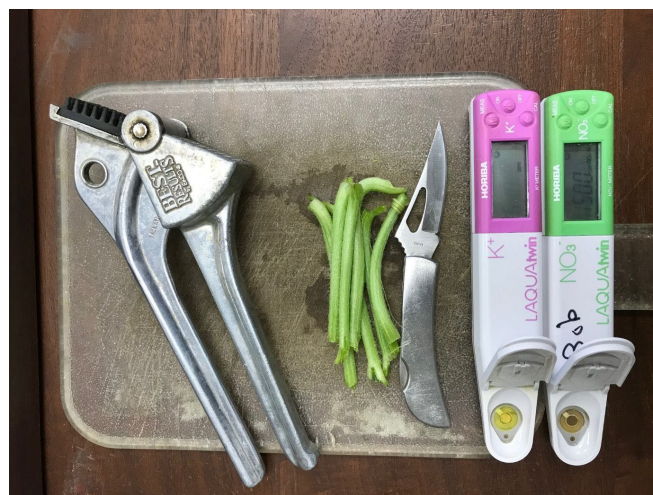
Figure 5. Horiba LAQUA twin meters for Nitrate-N and K with sample.
